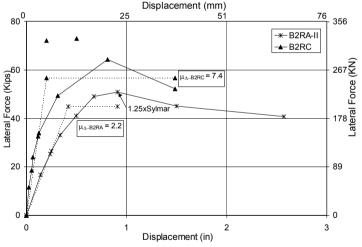
Figure 7 Comparisons of Force-Displacement Hysteresis Envelopes
