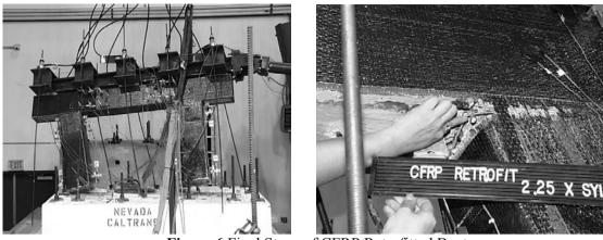
Figure 6 Final Stage of CFRP Retrofitted Bent
