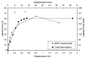
Figure 9 Force-Displacement Curve of the CFRP Retrofitted Bent
